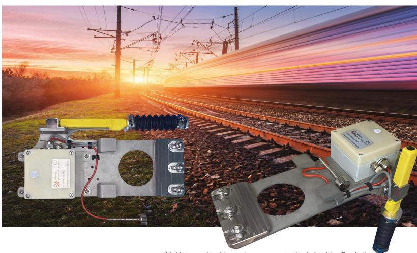
This internally powered dual sensor node allows remote measurement of dynamic distance displacement associated to track voiding and critical rail temperature (CRT) monitoring utilising a magnetic probe which measures the rail skin temperature.
