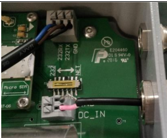
Figure. 110-240VAC to 12VDC@5A Adapter Connection.
