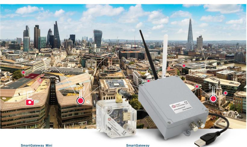
WiSenMeshWAN SmartGateway Mini is a mini-USB SmartGatewayfor WiSenMeshWAN sensor nodes. It manages the scheduling of the connected sensors and reads data from the node and transmits it to the local data server over USB connection. Locally stored data can be pushed to the Wisen cloud or imported immediately to 3<sup>rd</sup> party monitoring software. The SmartGateway Mini is directly powered from the USB connection.
